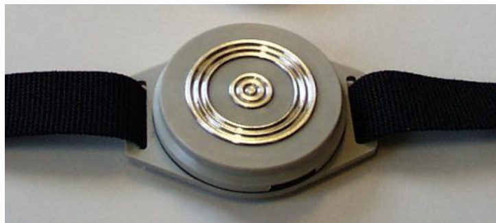
Figure 4.1: Combined SpO 2 , core body temperature and activity sensors with ECG and respiration electrode.
