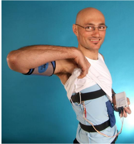
Figure 4.2: CSEM multi-parameter health monitoring system developed for the European Space Agency Long Term Medical Survey project at the Concordia Base Station in the Antarctica.
