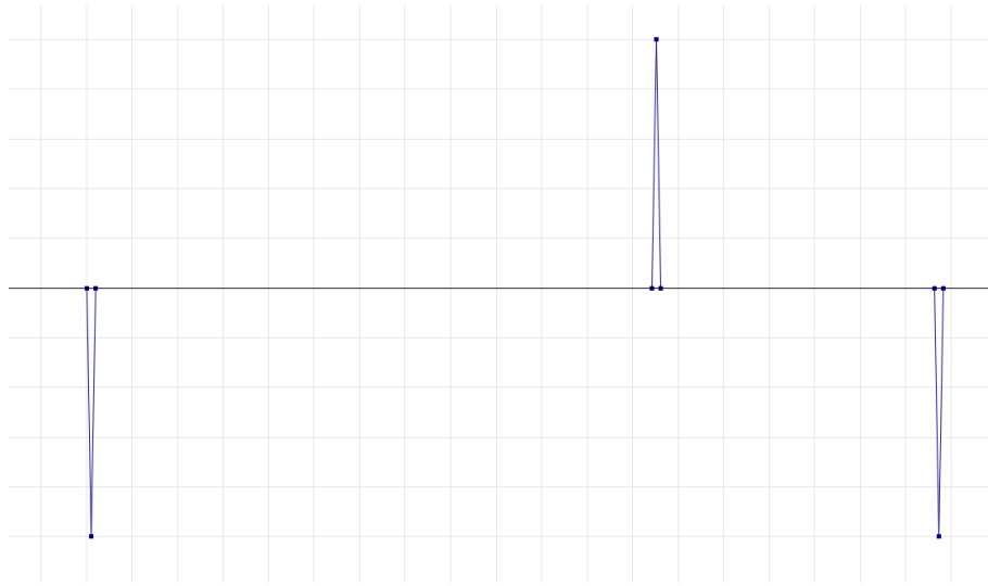
Figure 2.15: A few pulses of the IEEE 802.15.4A synchronization preamble as stored in the network simulator at the transmitter.
