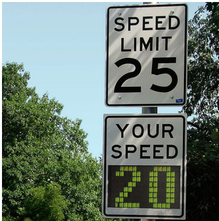
(a) Radar Speed Sign: Current speed vs. speed limit (Source: commons.wikimedia.org)
