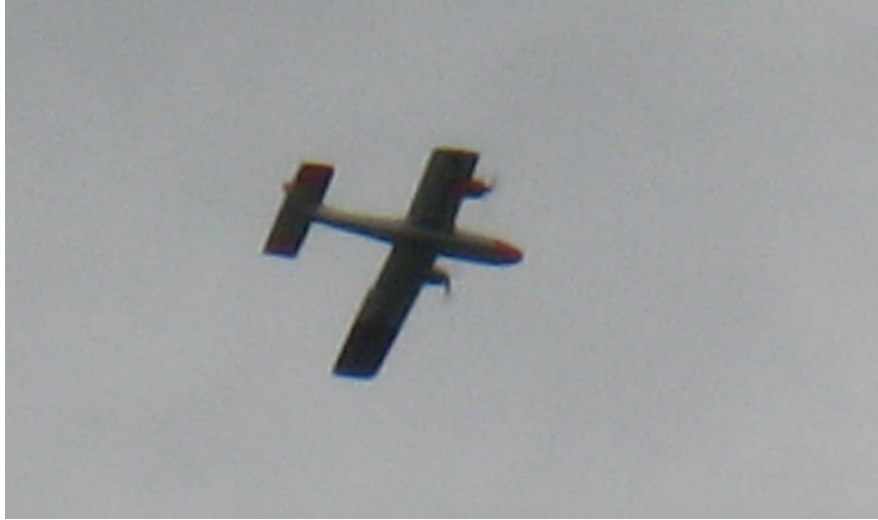
Figure 4 GT Twinstar in autonomous flight with 50% right wing failure
