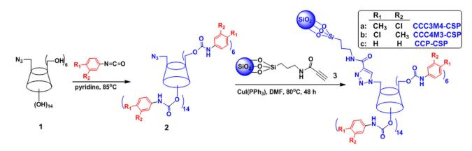
Figure 2. Click synthesis of perphenylcarbamated CD mono-clicked CSPs.
