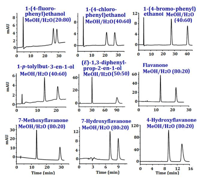
Figure 4. The representative enantioseparation chromatograms of selected analytes.
