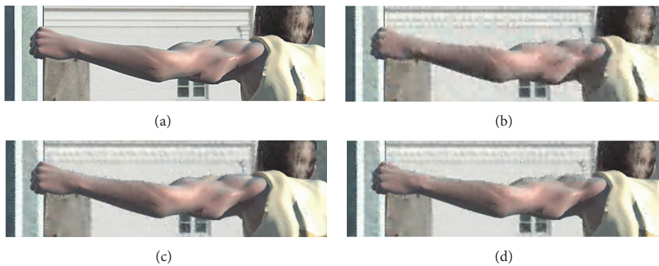
FIGURE 22: Zoom on visual quality of texture view for UndoDancer view 1 frame 250 (a) original, coded at 0.2bpp (b) by classic LAR (Global PSNR = 24 dB), (c) by applying the SNR quality enhancement ( Q_{p-Ref,T\_DoI} = 25 , Q_{p-Ref,T\_NDoI} = 120 ) using the full-resolution DoI-Mask of depth zone within Z_{in,l} = 100 and Z_{in,h} = 121 (Global PSNR = 28.82 dB, DoI coded at 0.98 bpp, PSNR_{DoI} = 36.06 dB, non-DoI coded at 0.17 bpp, PSNR_{Non-DoI} = 28.1 dB), and (d) by applying the SNR quality enhancement for 16 \times 16 block resolution DoI-Mask.
