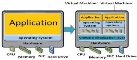
Figure 2. the architecture of computer device before and after virtualization
