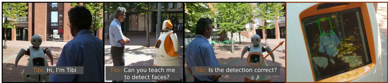
Fig. 1 Human-robot interaction and communication. Left: Tibi mobile robot approaches a person to initiate a conversation. Right: after the first contact, the person assists Tibi to improve its visual skills. A Wii's remote controller is used to help to validate and improve the visual face detector
