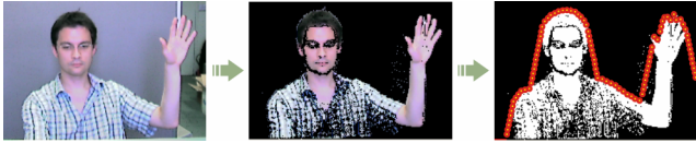
Figure 6. Gesture analysis. Left: input image. Center: background removal. Right: draping the outline.
