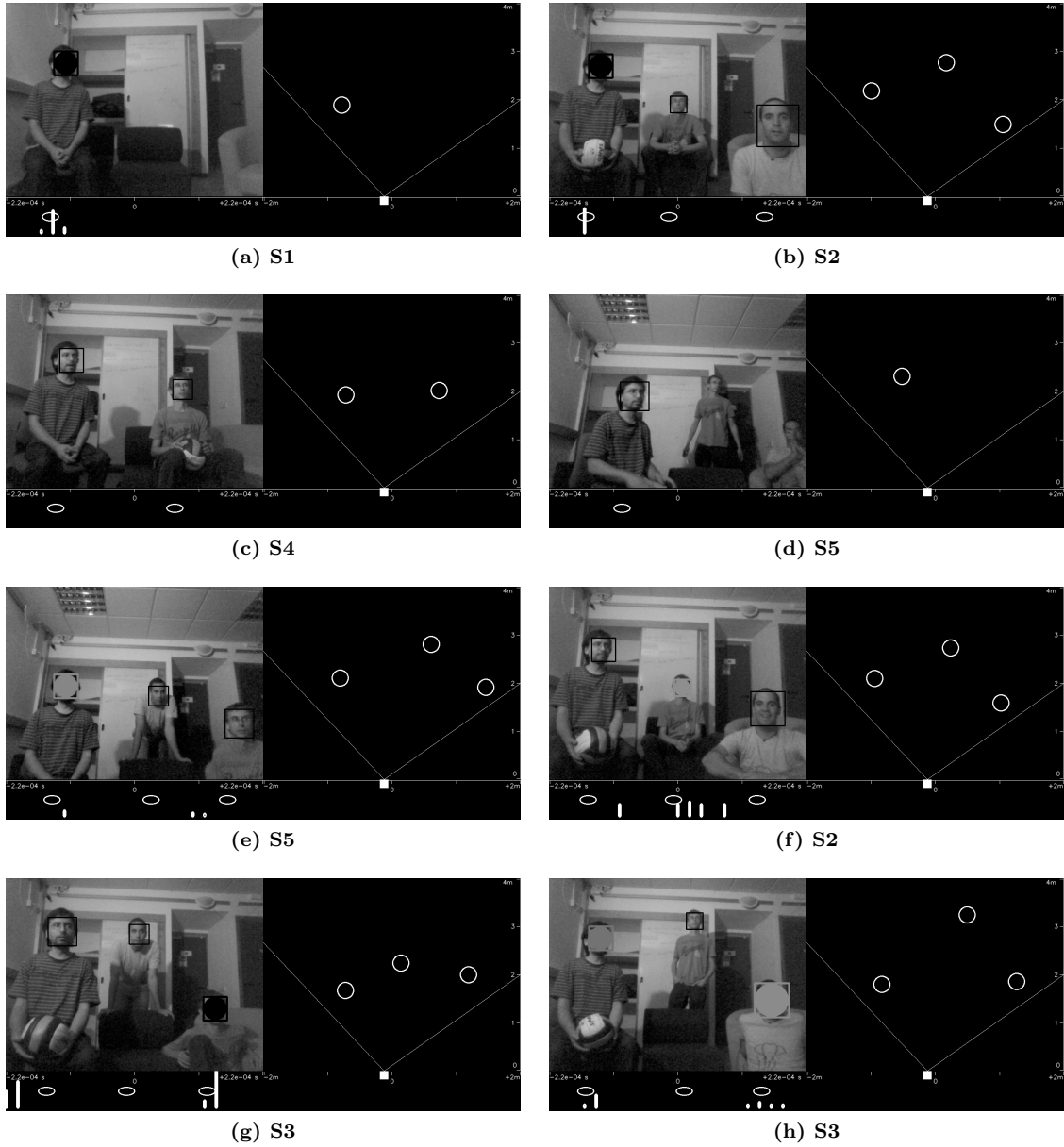
Figure 10: Snapshots of the visualization tool. Frames selected among the five scenarios to show the method's strengths and weaknesses. The faces' bounding box are shown superposed to the original image (top-left). The bird-view of the scene is shown in the top-right part of each subimage. The histogram of ITD values as well as the projected faces are shown in the bottom-left. See Section 6.3 for how to interpret the images above.
