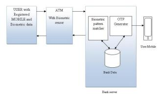
Figure 1. Block Diagram of securing ATM with OTP and Biometric
