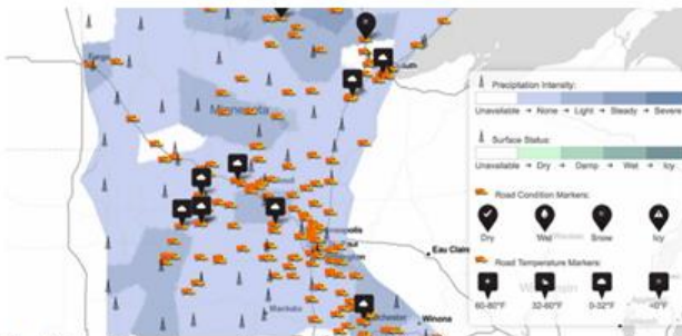
Traffic-related weather data. Weather, movement of snowploughs, and road conditions are shown during a snowstorm.
