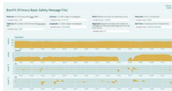
Interactive visual overview of the Basic Safety Message, that logs vehicle's attempt to communicate with roadside equipment.
