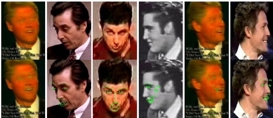
Figure 4-6 Some of the alignment results of SDM-based method [14] on the frames of the Youtube Celebrities database which are discarded by the proposed method due to excessively low face quality. The first row shows the low-quality face images and the second row shows the landmarks points detected by SDM.
