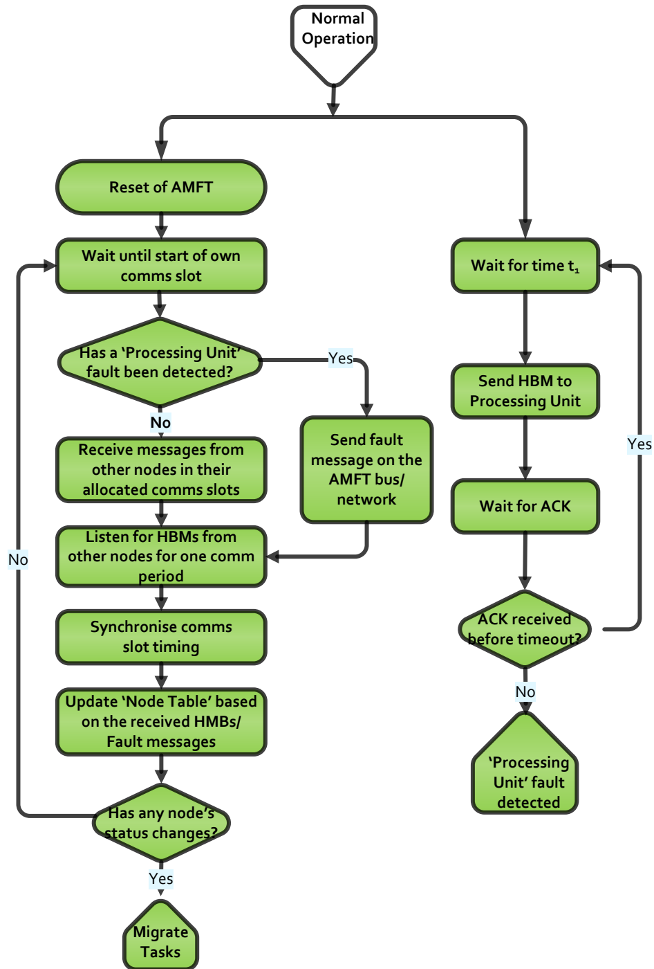
Figure 5.2: Algorithm for AMFT Normal Operations.
