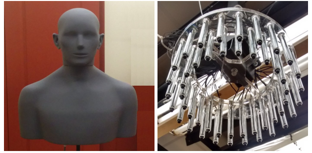
Fig. 2. The Cortex MK2 with built-in microphones at two ears and the 48-channel two-circular microphone array.
