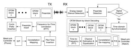
Fig. 3: The OFDM modem of WearLock.
