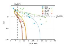
Fig. 5: The BER of different modulations changes with Eb/N0
