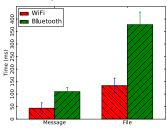
Fig. 11: The communication delay between smartphone and smartwatch.
