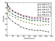
Fig. 4: Receiver's SPL in distance of different volume settings. Measured in a quiet room with the SPL of ambient noise about 15-20 dB in a line-of-sight scenario.
