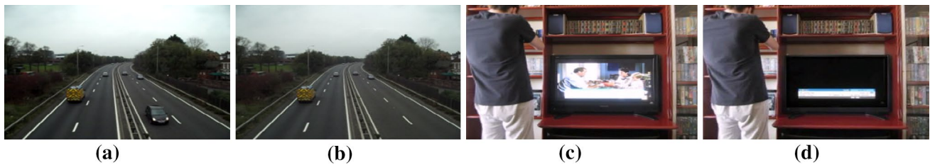
Fig. 1 Examples of copy–paste forgeries. a and c Represent sample frames from original videos [8], and b and d are their forged versions wherein certain objects have been removed
