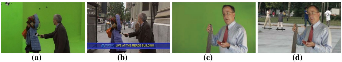
Fig. 4 Examples of green screening a and c represent sample frames of videos with people engaged in various activities in front of a green screen. b and d Frames from a new video where these people have been composited into their new surroundings [9, 10]
