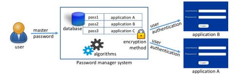
Fig. 1. Context of use and typical components of password managers.
