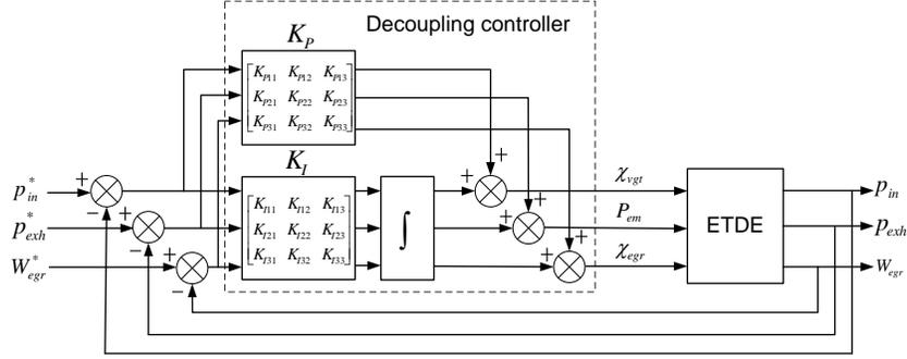
Figure 5: The diagram of ETDE air system control
