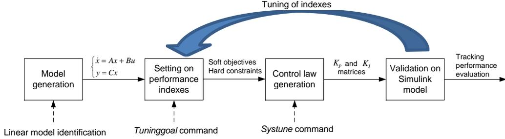
Figure 10: Workflow in developing low level controller
