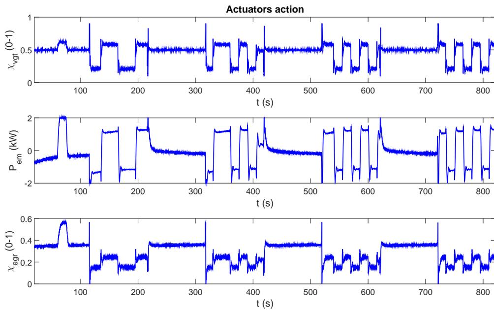
Figure 25: Actuator actions in two-level energy management test
