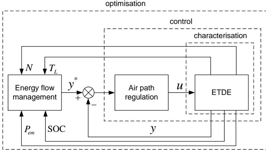
Figure 1: On-line energy management diagram of the ETDE
