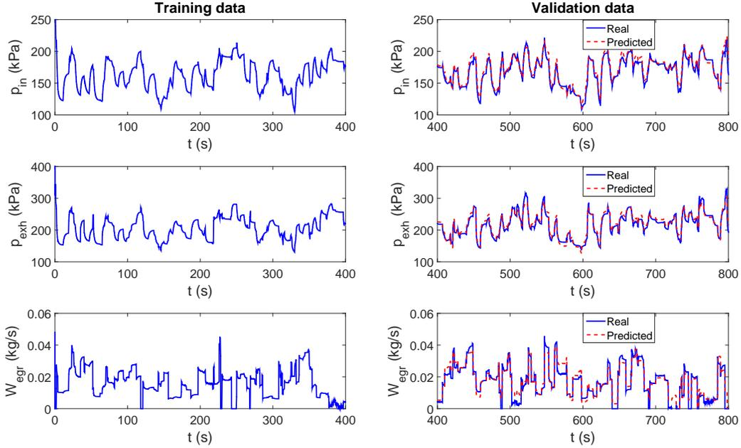
Figure 9: Training and validation in model identification
