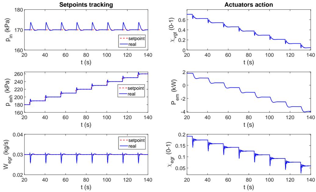
Figure 11: Mathematical simulation results at 1800 rpm, 260Nm
