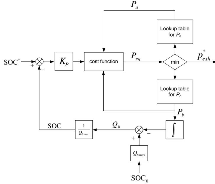
Figure 17: The diagram of supervisory level controller
