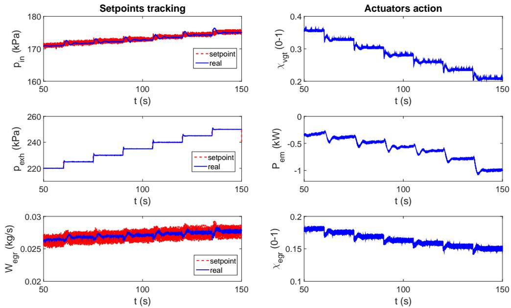
Figure 18: Physical simulation results at 1800 rpm, 260Nm
