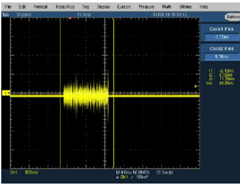
Fig. 8. OFDM signal output with high PAPR [57].
