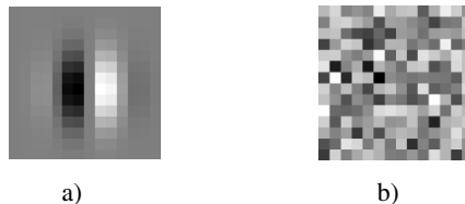
Fig. 2. Convolution kernels used for feature extraction. a) Imaginary part of 2D Gabor filter reached 99,058 % recognition accuracy. b) An example of the optimized kernel which reached 100% recognition accuracy.
