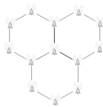
Fig 2: Antenna locations in tessellating hexagonal cells.
