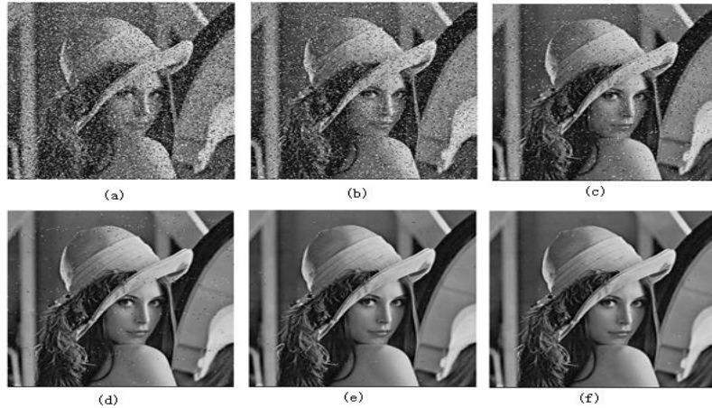
Figure 11. The result of image recovery with different signal noise ratio when iter=8. (a) The result of image recovery when the SNR=-0.5 dB.(b) The result of image recovery when the SNR=0 dB.(c) The result of image recovery when the SNR=0.5 dB.(d) The result of image recovery when the SNR=1dB.(e) The result of image recovery when the SNR=1.5 dB.(f) The result of image recovery when the SNR=2 dB.
