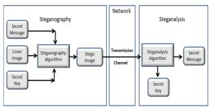
Figure 1: Steganography and Steganalysis Process
