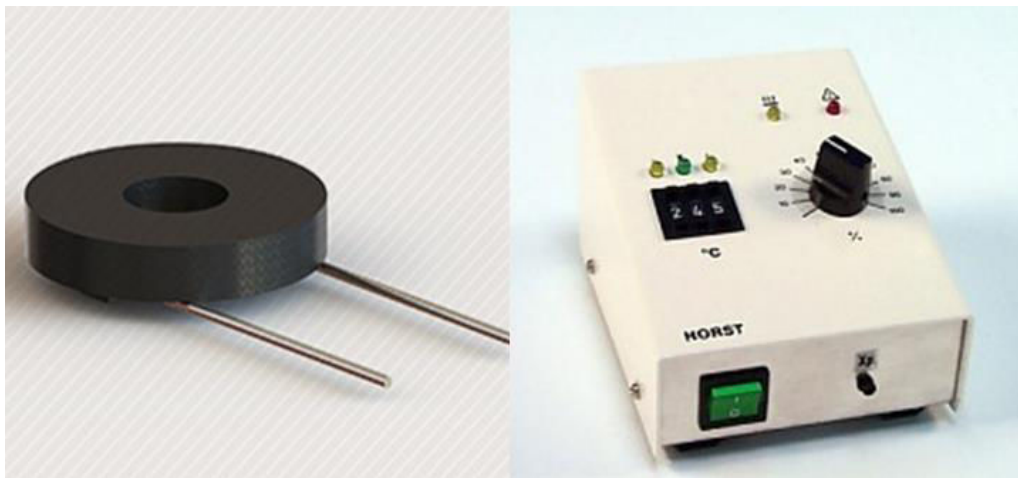
Figure 41: Resistive heater from Bach ceramics (left) and the temperature controller from Horst used to regulate the temperature. (Right)
