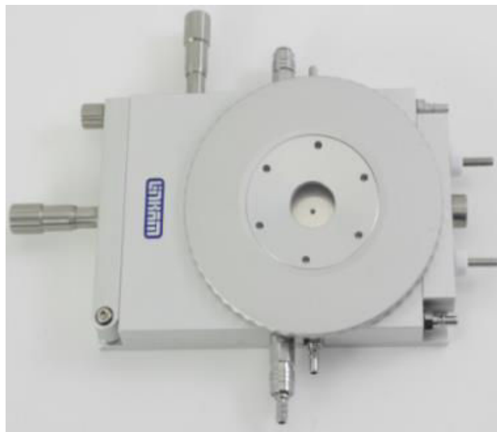
Figure 34: Photograph of a linkam stage with a glass opening for the laser to shine on the substrate.
