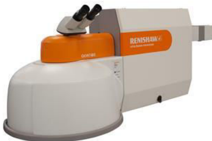
Figure 33: Photograph of the Renishaw in via Raman spectrometer.
