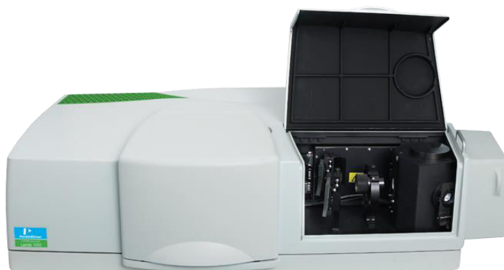
Figure 40: Photograph of the spectrophotometer by Perkin Elmer with a 150 mm integration sphere.
