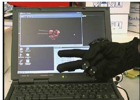
FIGURE 2 Data glove based system
