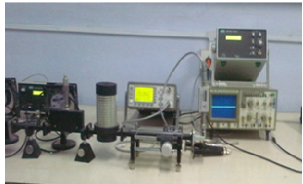
Fig.2 Power Loss measurement setup
