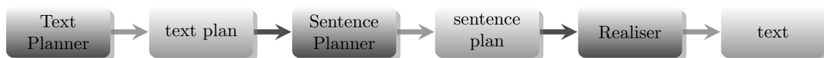
Figure 3: Classical three-stage NLG architecture, after Reiter and Dale (2000). Darker segments illustrate the three main modules; lighter segments show the outputs.
