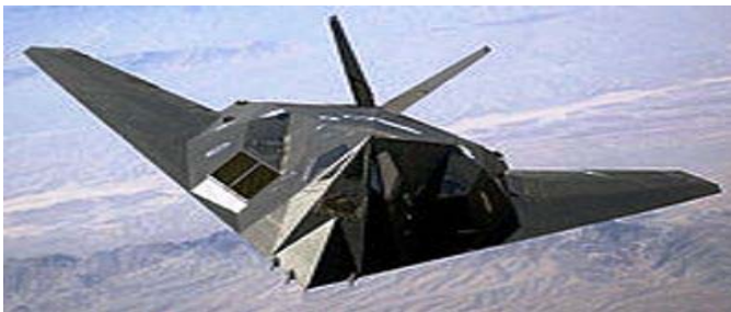
Fig.7. Stealth Aircraft uses Iron Ball Paint
