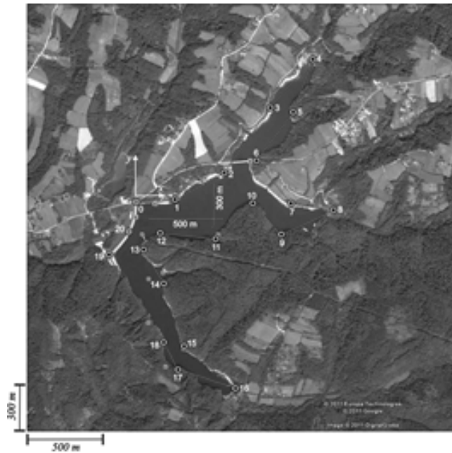
Figure 5. Google-Earth map of the lake used to define desired GPS trajectory of the quad-rotor flying robot.
