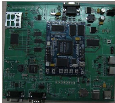
Figure 10. Development board based on new high secure architecture of network computer
