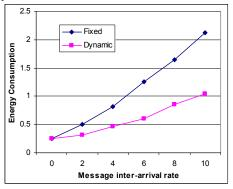
Fig. 5: Energy consumption as a function of message inter-arrival period when fixed cluster heads and dynamically changing cluster heads used.
