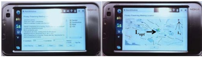
Figure 7. Prototype POML application running on a Nokia N810 mobile device. The image on the left is the main window, where users add the desired meeting participants. The image on the right is the map that shows the optimal meeting location (green pin, thick solid arrow) and the user-desired meeting location (red pin, thin dashed arrow), after the execution of the POML protocol. In this particular example, the optimal meeting location is not this user's preferred location, but the location preference of some other participant.
