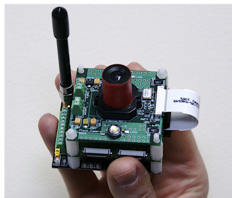
Fig. 1: Illustration of camera stack formed by a Fleck sensor node, DSP board and CCD camera.
