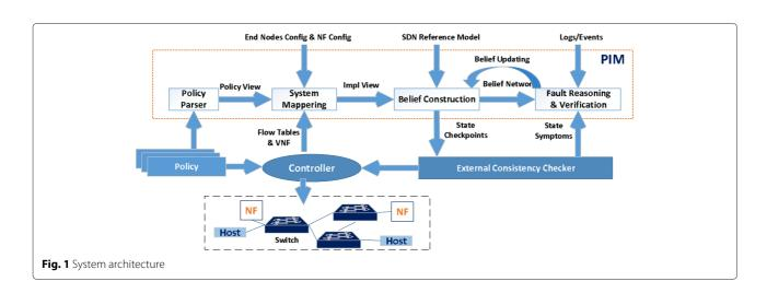
pair of logical end nodes, traffic pattern specification, and a list of required network functions (or a service function chain). Network Functions are required mainly for meeting with various requirements in network connectivity, security and performance.
