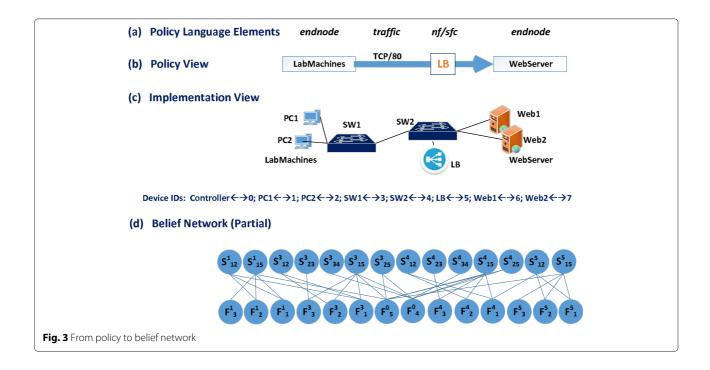
(e.g., LB) onto the plumbing graph, and then identify the necessary pipe(s) (i.e., the network topology for this service) connecting all these endnodes and NF nodes. The *Implementation View* renders the service topology with all related nodes (e.g., endnodes, NF nodes) and the intermediate forwarding switches as an example shown in Fig. 3c.
