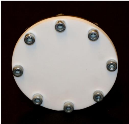
Fig. 1: First prototype of the SAW transponder covered in a protective housing to resist the hot sulfuric acid.
