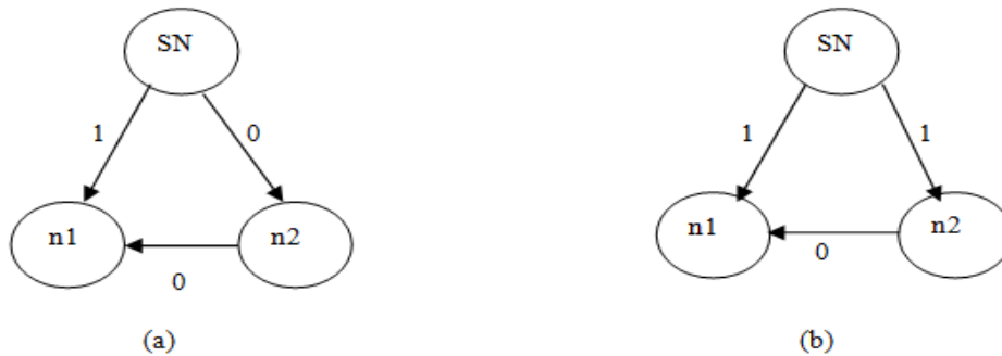
Fig 1. (a) The Case where source node is faulty (b) the case where participant node is faulty
