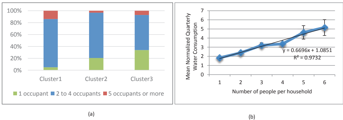
Fig. 3. “HOUSEHOLD” case study: (a) Cluster analysis and (b) plot and linear regression of water consumption vs. number of occupants in household.
