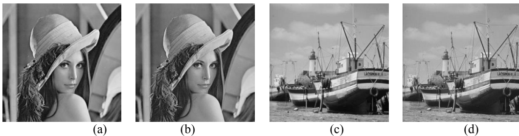
Fig.4. (a) cover image (b) stego image with capacity 250,343 bits and PSNR 34.096 dB (c) cover image (d) stego image with capacity 233,918 bits and PSNR 31.604 dB
