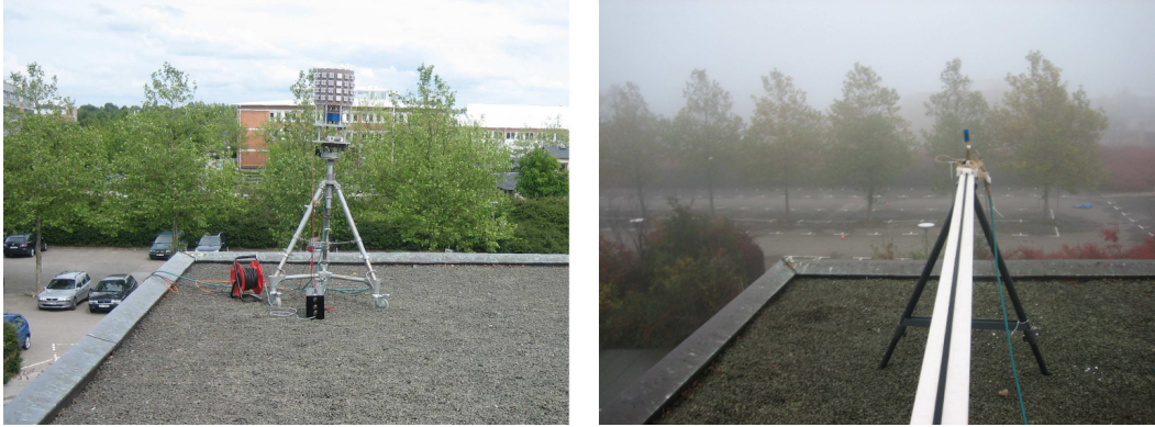
Figure 5: Massive MIMO antenna arrays used for the measurements.
