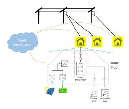
Fig. 1. Powernet's deployment within the legacy grid.
