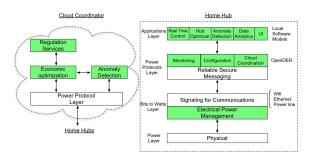
Fig. 2. Logical layering of required functionalities.
