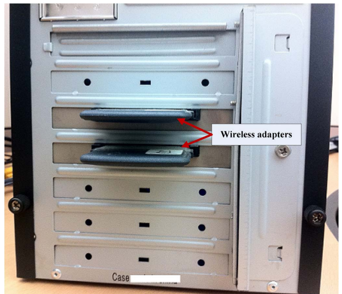
Fig. 2. Test bed equipped with two wireless adapters.
