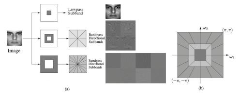
Fig. 1. Nonsubsampled contourlet transform: (a) NSFB structure and (b) idealized frequency partitioning obtained by NSFB.
