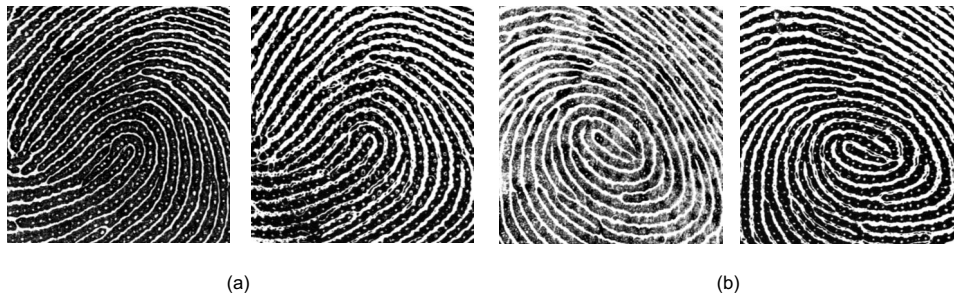
Fig. 6 Two sets, (a) and (b), of live and fake fingerprint images captured with a 1000-dot/in. high-resolution optical sensor (CrossMatch Co. Ltd). Left: live image; right: corresponding fake image.
