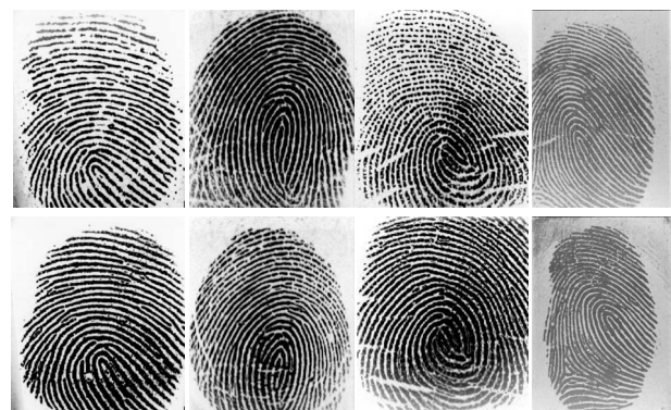
Fig. 10 Some examples of live and fake fingerprint images obtained from the four sensors: live fingerprint images (top row) and their corresponding fake fingerprint images (bottom row).
