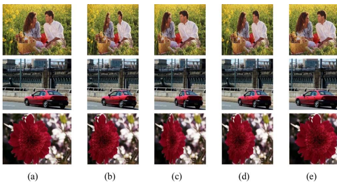
Fig. 13. Retargeted image samples from the first image dataset (images with complex background) for four algorithms. (a) Original images. (b) Retargeted images from [29]. (c) Retargeted images from [30]. (d) Retargeted images from [16]. (e) Retargeted images from our algorithm. The sizes of the original images and the retargeted images are 300 \times 400 and 300 \times 300 , respectively.
