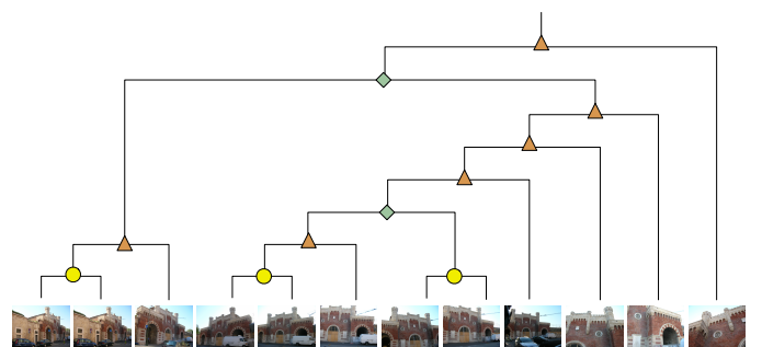
Figure 3: An example of a dendrogram for a 12 image set. The circle ● corresponds to the creation of a stereo-model, the triangle ▲ corresponds to a resection-intersection, the diamond ◆ corresponds to a fusion of two partial independent models.
