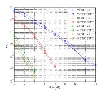
**Figure 8.** Performance comparison of the system with STBC based STTC and B-STTC based STBC site diversity techniques for various antennas
