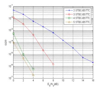
**Figure 6.** Performance of the system with STBC based B-STTC site diversity for various antennas
