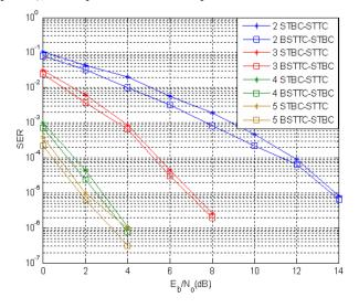
**Figure 7.** Performance comparison of the system with STBC based STTC and B-STTC based STBC site diversity techniques for various antennas
