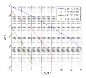
Figure 5. Performance of the system with B-STTC based STBC site diversity for various antennas
