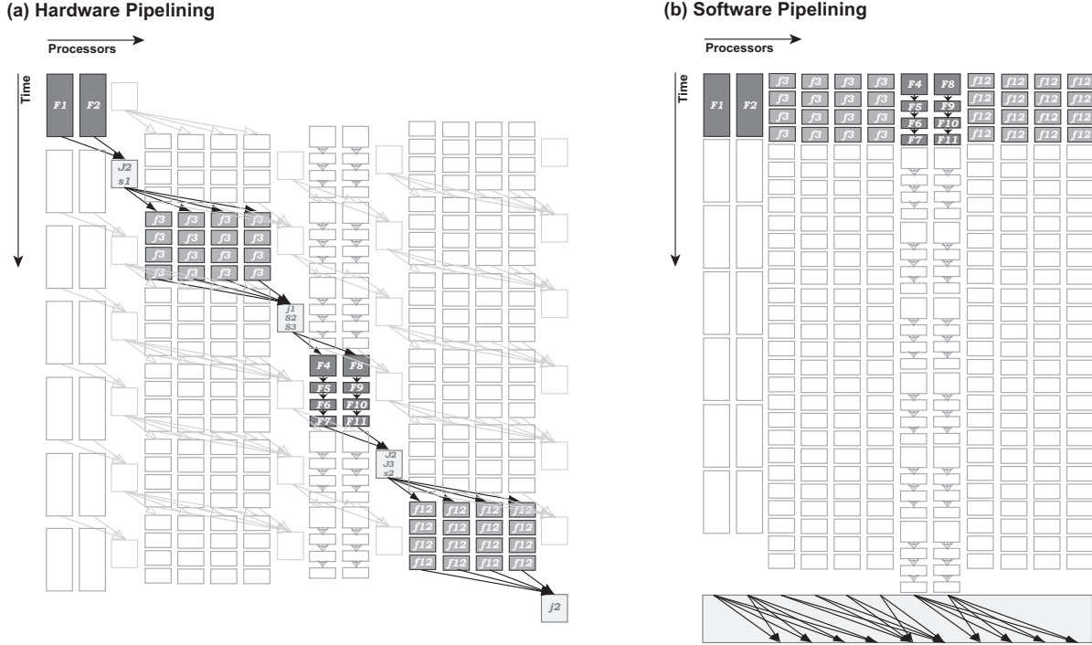
Figure 5. Comparison of hardware pipelining and software pipelining for the Vocoder example (see Figure 1). For clarity, the same assignment of filters to processors is used in both cases, though software pipelining admits a more flexible set of assignments than hardware pipelining. In software pipelining, filters read and write directly into buffers and communication is done at steady-state boundaries. The prologue schedule for software pipelining is not shown.
