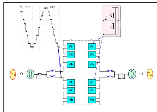
Fig.1 Typical structure of MMC-HVDC
