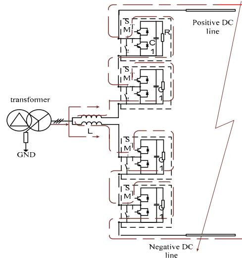
Fig.6 Current direction after dc short circuit occurred
