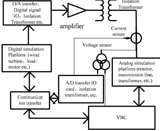
Fig.4 Interface of digital and analog subsystem
