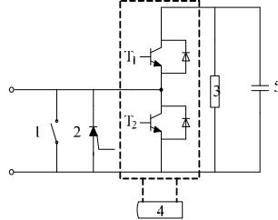
(1.bypass switch, 2. thyristor, 3.parallel resistors, 4.SMC, 5.capacitor)
