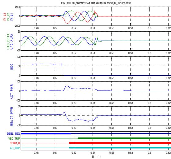
Fig.9 Waveform of protection after shortout occurs
