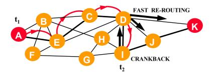
Fig. 10. Illustration of crankback and fast-rerouting.
