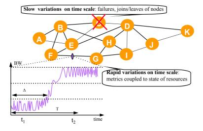
Fig. 8. Network topology changes on different time scales
