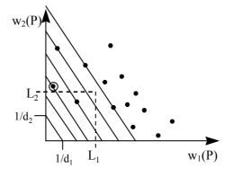
Fig. 1. Representation of the link weight vector  $\boldsymbol{w}(P)$  in two dimensions. The dotted rectangle spanned by the constraints  $L_1$  and  $L_2$  forms the space of feasible paths. Jaffe's scanning procedure first encounters the encircled node, which is the path with minimal length.
