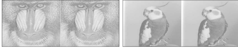
Fig. 5. Fidelity Performance of the Proposed Scheme: (from left to right) Original Baboon Image Data Embedded Baboon with PSNR = 34.8704, Original Bird Data Embedded Bird with PSNR = 53.76
