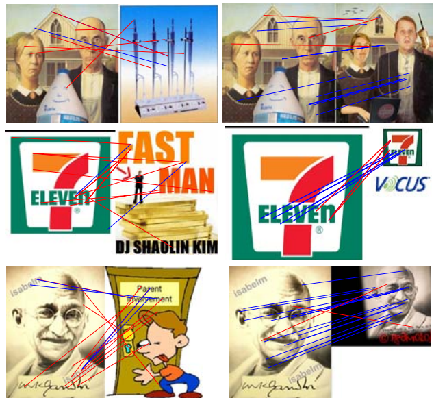
Figure 6. Matching results verification by binary SIFT ( t = 18 ). The initial matches are obtained by vector quantization with VW 500K. Red line: false matches identified by binary SIFT verification; blue lines: true matches passing matching verification. (left) irrelevant image pairs; (right) relevant image pairs. (Best viewed in color PDF)
